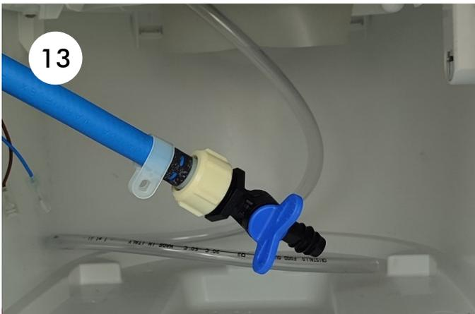
13. Close the fresh water hose with the ball valve. We recommend opening the fresh water hose once a month and flushing it with water.
