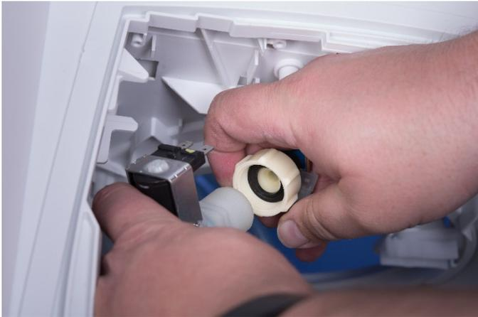
12. Disconnect the fresh water hose from the fresh water pump. Have a bucket ready to collect water standing in the hose.
