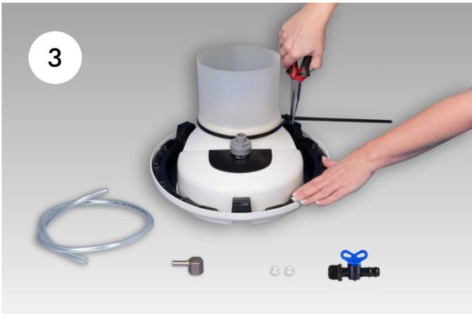
3. Tighten the cable tie using the needle-nose pliers. To do so, place the pliers directly behind the head of the cable tie and turn them anticlockwise.
