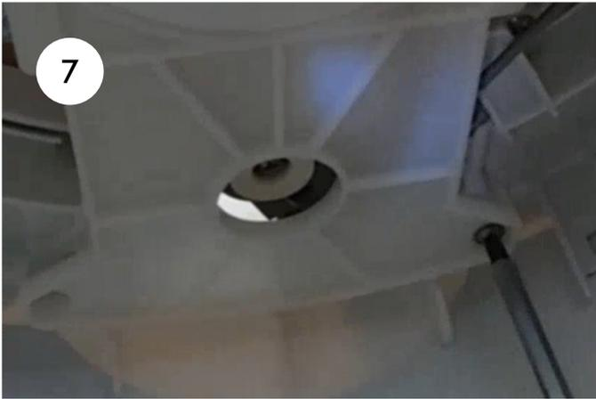
7. Through the service flap, loosen the four screws of the two clamps that secure the seat part of your Thetford chemical toilet to the base. Then pull the clamps off in a clockwise direction.
