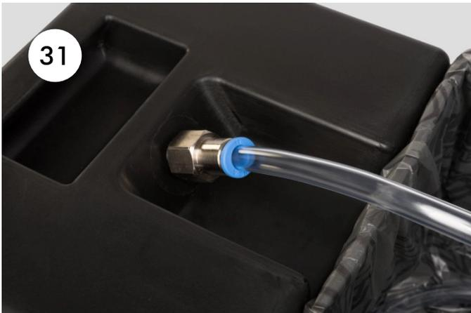
31. Insert the hose into the hose connection of the cassette. Check that it is in tight contact with the silicone sleeve and that there are no kinks, beads and that it has a downward slope. If this is not the case, you should shorten the hose again by a few mm.
