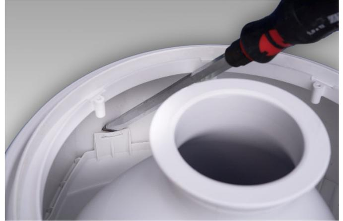
16. Loosen the bowl by carefully pushing one of the two rear fastening clips forward with a screwdriver with a long shaft. If the bowl still does not pull off well, loosen the second rear fastening clip in the same way.
